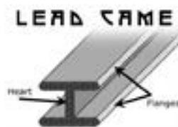
Fig.3. Cross section of lead caming; glass inserts in the groove. Zinc caming is hollow instead of solid, and lighter and more rigid.
