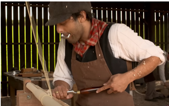
Abby turning a chair leg at the pole-lathe while playing his harmonica
